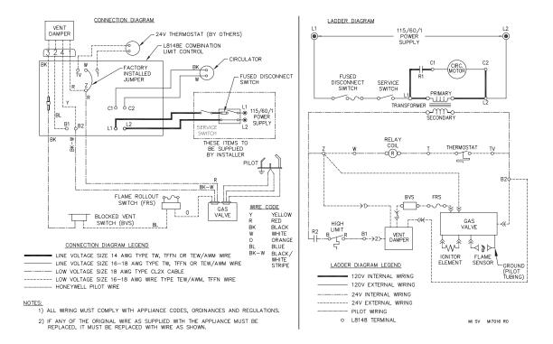
Figure 6.3: Wiring and Connection Diagram - Intermittent Ignition
